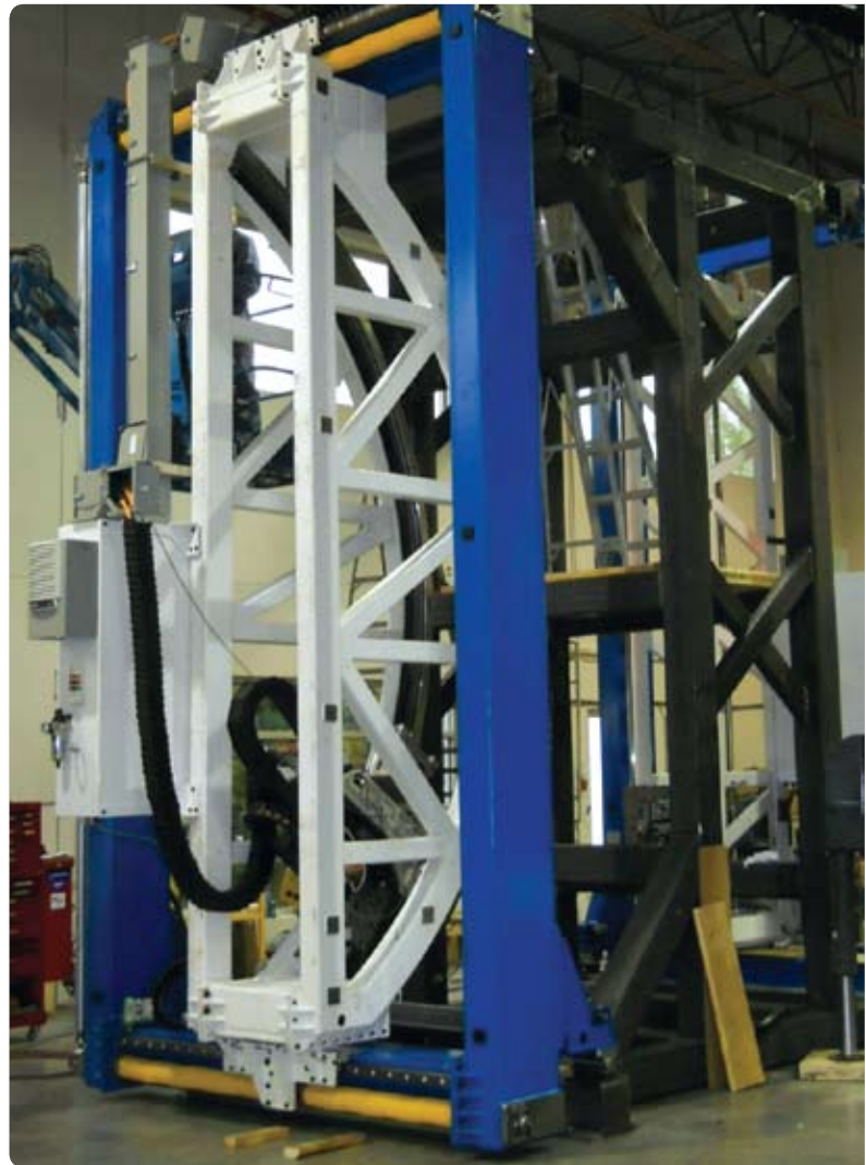
FIGURE 12 Airbus A350 Keel Beam Curved NC Drilling Machine
