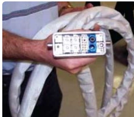
FIGURE 10 📌 Flex Track Umbilical that delivers high/low voltage, compressed air, and data to machine
