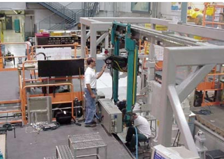
FIGURE 13 NCDJ 5-axis drilling machine used to drill F/A-18 forward fuselage.
