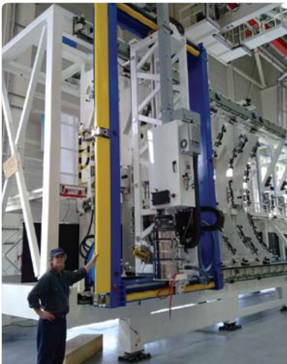
FIGURE 16 📍 A350 Keel Beam NC Drilling Machine
