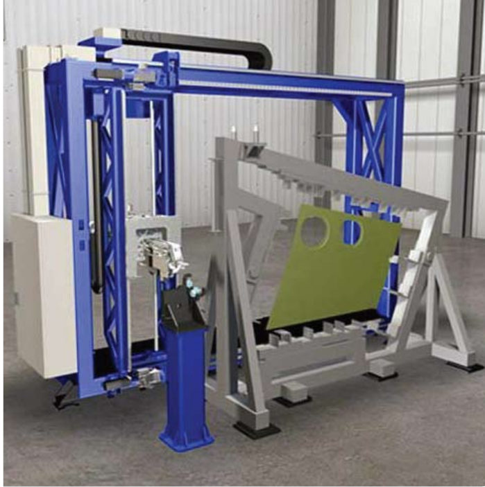
FIGURE 15 📍 Boeing F/A-18E/F outer wing NCDJ machine concept
