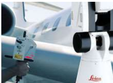
Aerospace manufacturers use Leica's laser tracker portable CMMs for measurement of large aircraft structures.
