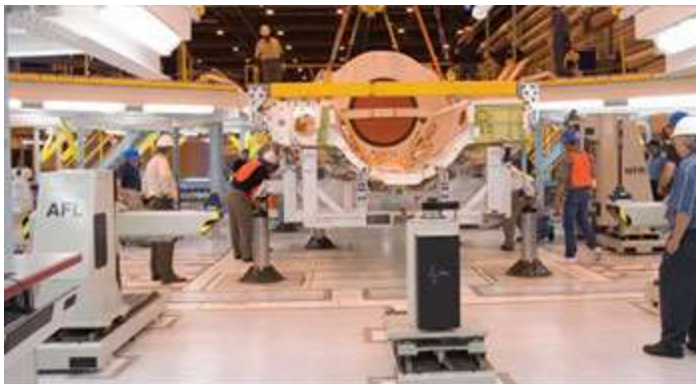
Using Leica's Laser Trackers, Lockheed Martin employs its laser-guided Electronic Mate and Alignment System (EMAS) to join large aircraft components including the fuselage and wings for the F-35 fighter plane. Photo courtesy Lockheed Martin Corp.
